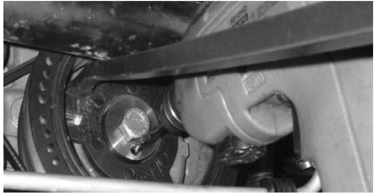
Pinning Tool Installation (Factory Balancer Shown)
