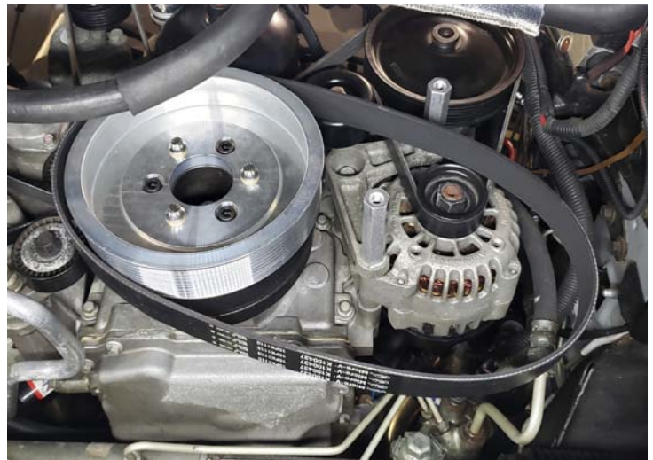
Belt Loosely Installed
