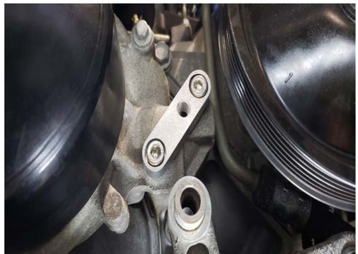
Sub Bracket Installed
