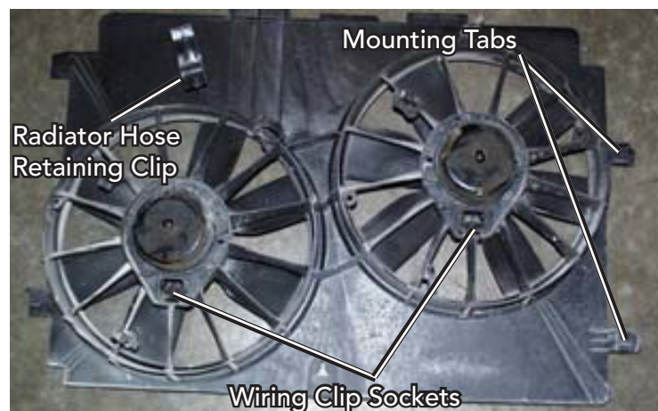
Factory Fan/Shroud Assembly (Removed)
