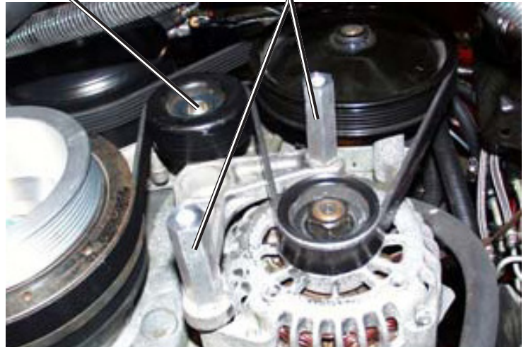
Main Bracket Standoffs Installed
