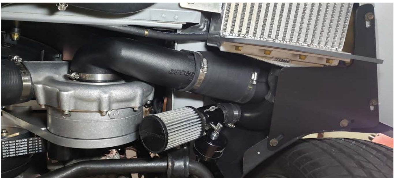
Surge Valve Assembly Installed
