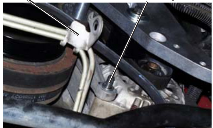
Transmission Cooler Lines & Securing Tab
