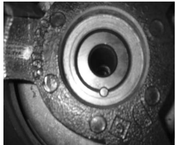
Harmonic Balancer Pinned to Crankshaft
