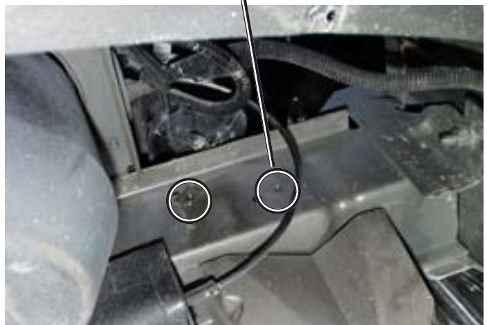
Horn Relocation Holes (Shown with Horns Removed)
