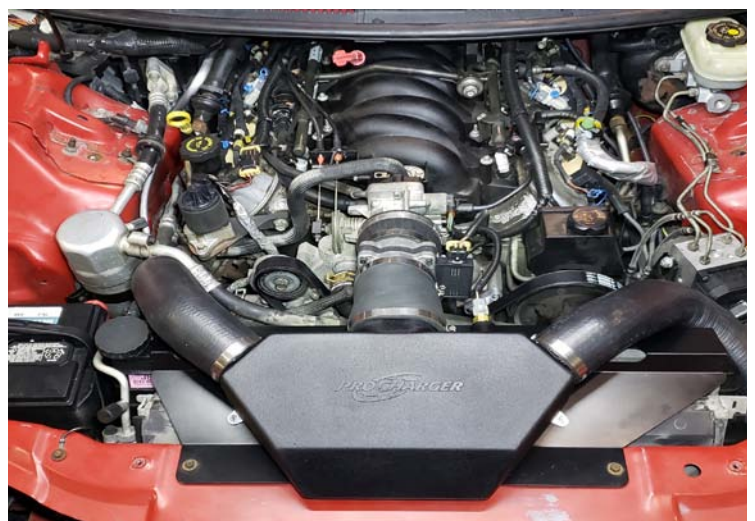
Rotomold Plenum Installed
