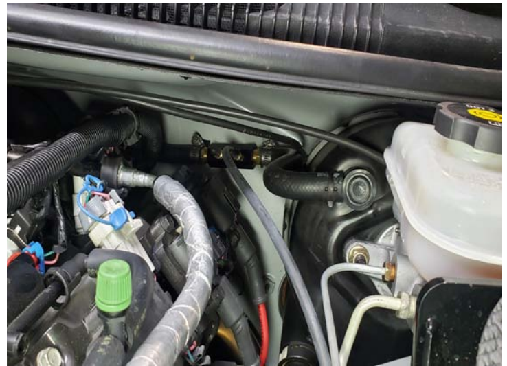
Vacuum Manifold Installed
